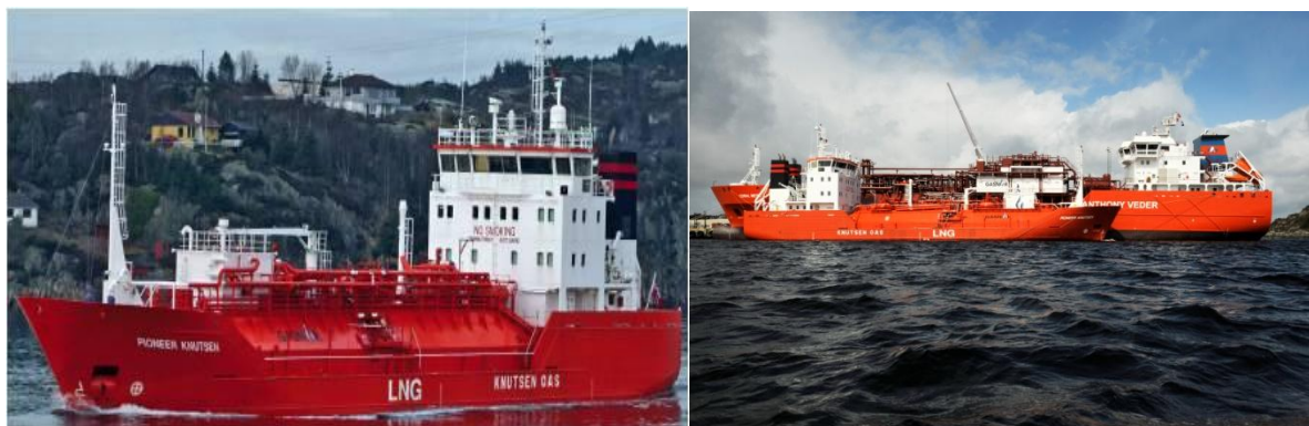
Figure 19 Small scale pressurized tank LNG ships (1100m 3 Pioneer Knutsen & 7500m 3 Coral Methane), Source: Shell, Knutsen and Anthony Veder.
