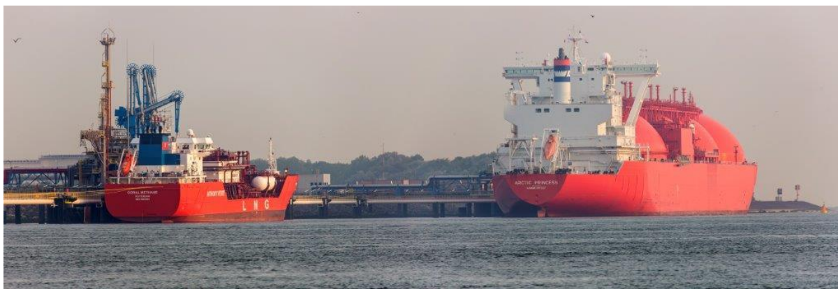
Figure 20 Small Scale Vessel Coral Methane 15.000m 3 and Arctic Princess conventional LNG carrier at Gate Terminal. Source: GATE Terminal, Rotterdam via Vopak.
